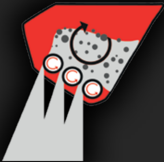
PHASE 2 » Screening & Crushing of material » Normal drum rotation » Optimal material flow and circulation » Minimal vaulting » Approx. 2/4 of full bucket
