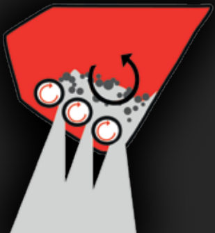
PHASE 3 » Reversed drum rotation » Approx. 1/4 of full bucket
